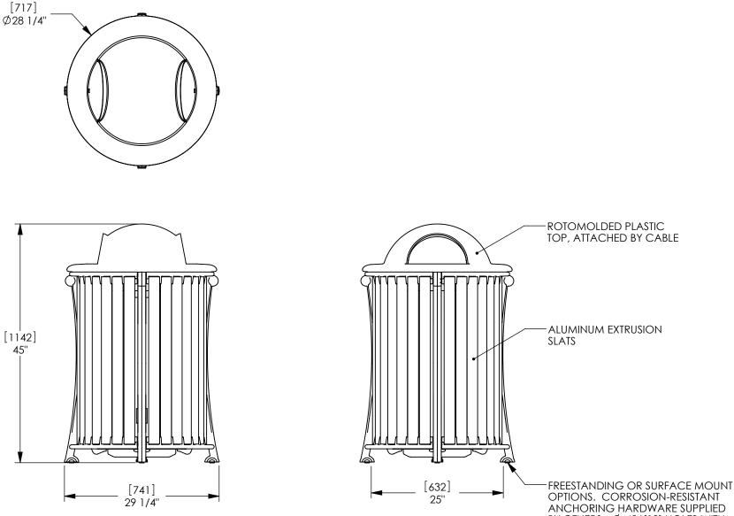
OPTIONS. CORROSION-RESISTANT ANCHORING HARDWARE SUPPLIED BY OTHERS. Ø.406[10] HOLES WITH COUNTERBORE PROVIDED FOR SOCKET HEAD CAP SCREWS.
